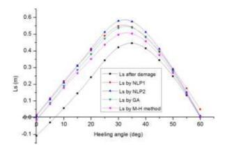
Fig. 3. Static stability curve by different method
